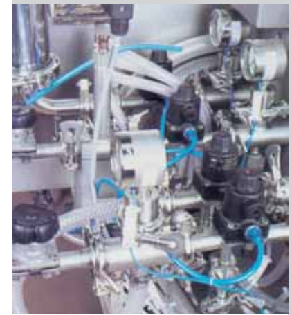
Picture 6.3: Flaps, valves with iglidur® X, high temperatures
