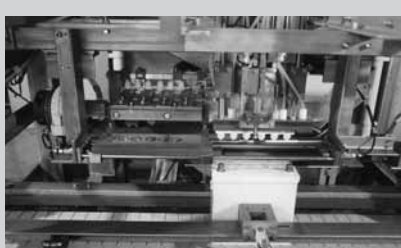
Picture 6.2: Battery filling
