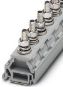
High Current Connectors, Connection method: Bolt connection, Cross section: 2.5 mm 2 - 95 mm 2 , AWG: 14 - 3/0, Width: 24.5 mm, Color: gray, Mounting type: NS 35/7,5
