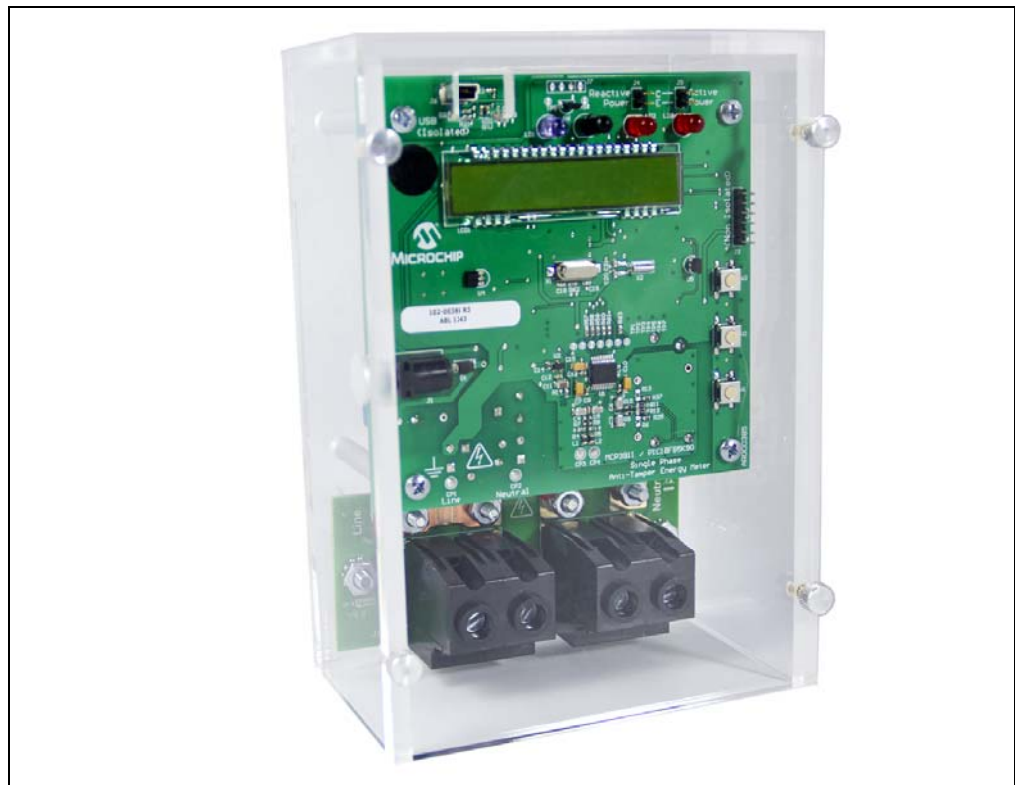
FIGURE 1-1: MCP3911 and PIC18F85K90 Single-Phase Anti-Tamper Energy Meter Reference Design.
