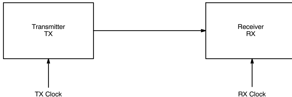
Figure 33. Example of a Serial Data Transmission System
