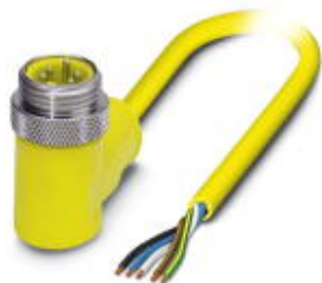
Sensor/Actuator cable, 5-position, PVC, Yellow RAL 1021, Plug angled 7/8"-16UNF, A-coded, on free cable end, Cable length: 2 m
