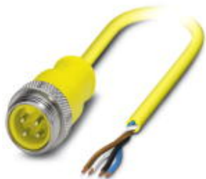
Sensor/Actuator cable, 4-position, PVC, Yellow RAL 1021, Plug straight 7/8"-16UNF, A-coded, on free cable end, Cable length: 2 m
