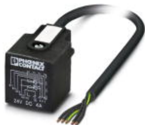
Sensor/Actuator cable, 5-position, PVC, Black RAL 9005, free cable end, on Valve connector AD (pressure switch), with 2 LEDs, Cable length: 10 m
