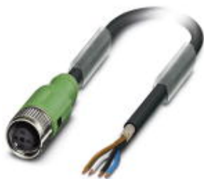
Sensor/Actuator cable, 4-position, PUR halogen-free, black-gray RAL 7021, shielded, free cable end, on Socket straight M12 SPEEDCON, A-coded, Cable length: 3 m
