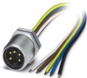
Sensor/actuator flush-type plug, 5-pos., 7/8", rear mounting with 7/8" fastening thread, with 1.0 m PE litz wire, 5 x 0.75 mm 2
