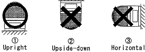
Mounting direction in outdoor (Please use a rubber mount)
