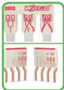
Two staggered jumpers 1 - 3 - 5 - 7 Staggered for use in a jumper slot Locate red stripes of the staggered jumpers on the inside
