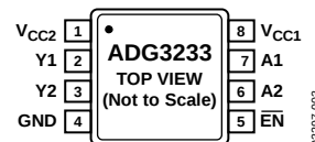
Figure 6. 8-Lead MSOP Package (RM-8)
