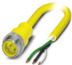
Sensor/Actuator cable, 3-position, PVC, Yellow RAL 1021, Plug straight 7/8"-16UNF, A-coded, on free cable end, Cable length: 2 m
