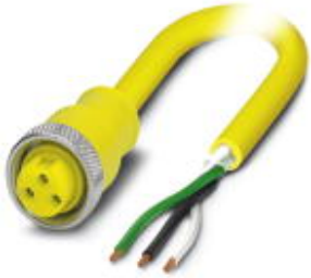
Sensor/Actuator cable, 3-position, PVC, Yellow RAL 1021, free cable end, on Socket straight 7/8"-16UNF, A-coded, Cable length: 6 m
