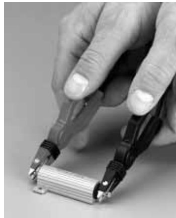
Four-wire measurement with only two clamps.
