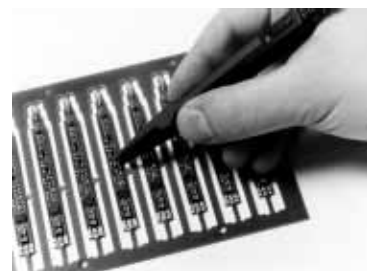
Test tweezers for extremely fine test connections
