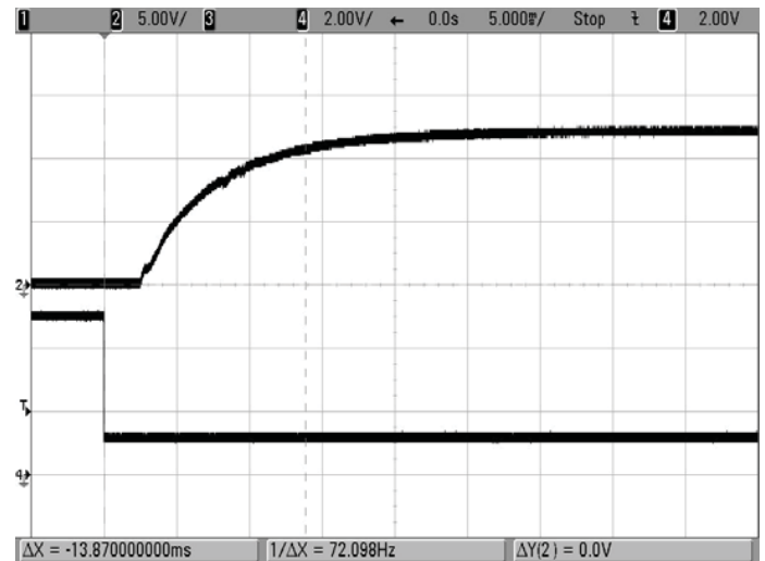
Enable Start-up ( V_{IN}=48V , I_{OUT}=5A , C_{LOAD}=1000\mu F , T_a=+25^\circ C ) Trace 2=Output, Trace 4= Enable.
