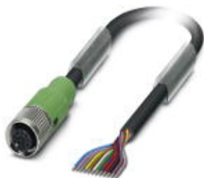
Sensor/Actuator cable, 12-position, PVC, Black RAL 9005, free cable end, on Socket straight M12 SPEEDCON, A-coded, Cable length: 3 m
