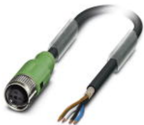
Sensor/Actuator cable, 4-position, PUR halogen-free, black-gray RAL 7021, shielded, free cable end, on Socket straight M12 SPEEDCON, A-coded, Cable length: 10 m
