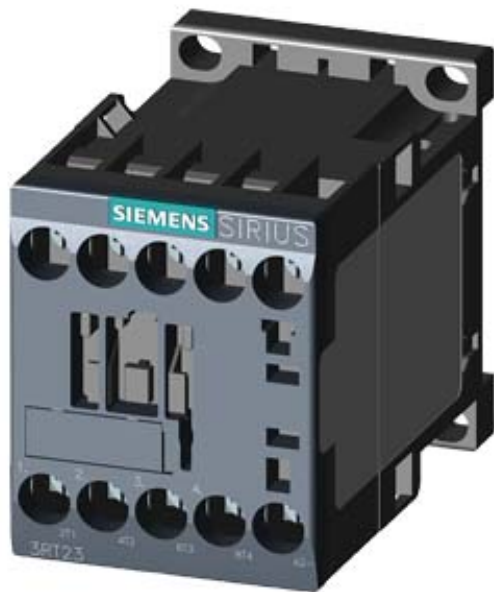
4NO CONTACTOR, AC1: 18A DC 24V 4-POLE, 4NO, SZ: S00, SCREW TERMINAL
