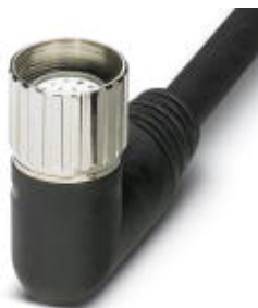
Female connector, Number of positions: 19, Status indication: No; Master cable connection: M23 socket, Cable length: 5 m, Shielding: No
