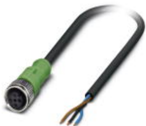
Sensor/Actuator cable, 3-position, PVC, Black RAL 9005, free cable end, on Socket straight M12, A-coded, Cable length: 10 m
