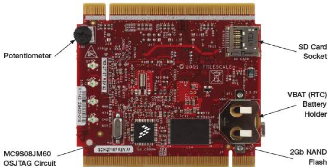
Figure 3. Callouts on back side of the TWR-K60F120M
