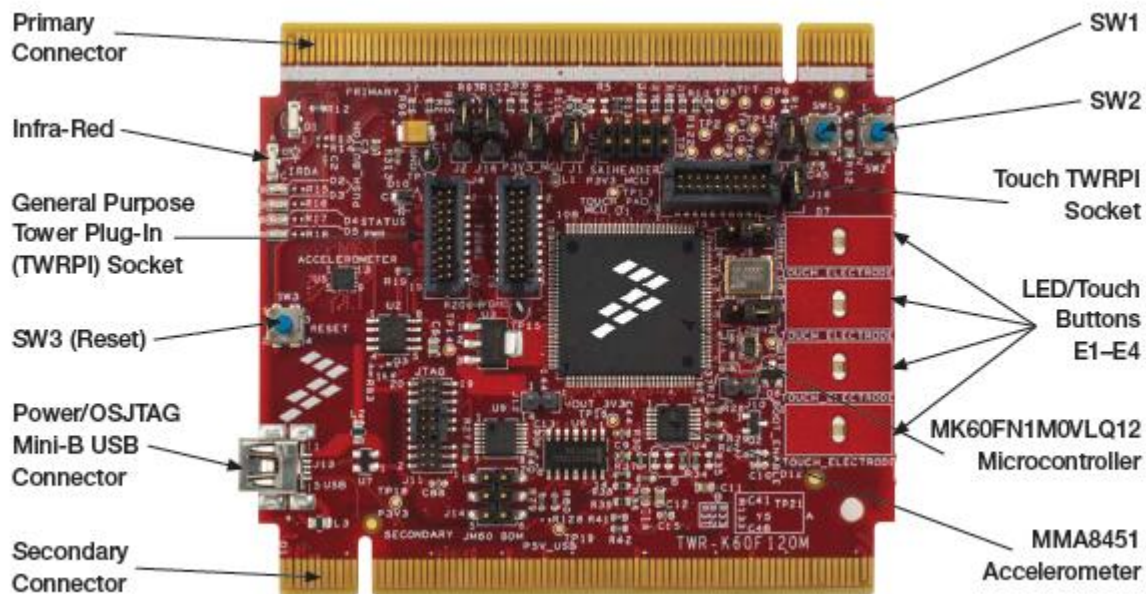
Figure 2. Callouts on front side of the TWR-K60F120M
