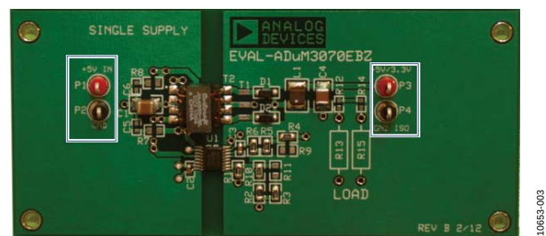
Figure 3. Single Supply Terminals
