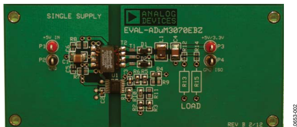
Figure 2. Single Supply Configuration
