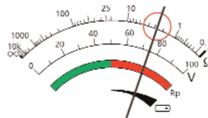
Figure 15: Resistance reading between 'X' and 'Y' terminals
