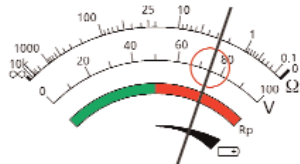
Figure 14: Analogue display indicating ground noise voltage measurement
