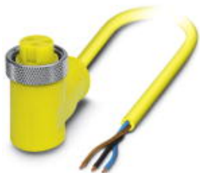
Sensor/Actuator cable, 3-position, PVC, Yellow RAL 1021, free cable end, on Socket angled 7/8"-16UNF, A-coded, Cable length: 2 m
