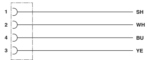
Contact assignment of the M12 socket
