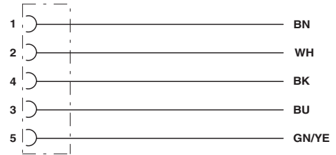
Contact assignment of the M12 sockets
