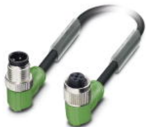
Sensor/Actuator cable, 3-position, PUR halogen-free, black-gray RAL 7021, Plug angled M12, A-coded, on Socket angled M12, A-coded, PIN 2+4 bridged, Cable length: 3 m
