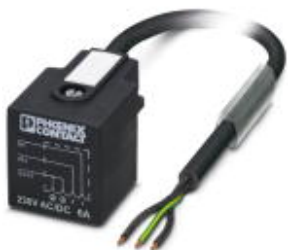
Sensor/Actuator cable, 3-position, PUR halogen-free, black-gray RAL 7021, free cable end, on Valve connector A, Cable length: 5 m
