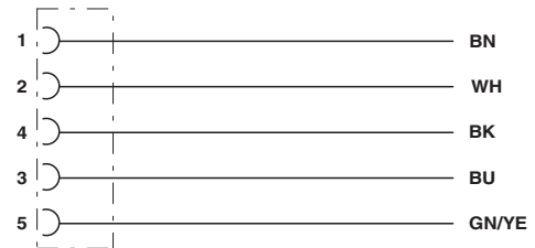
Contact assignment of the M12 sockets
