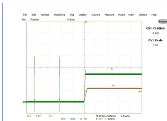
Figure 35: Short Circuit Recovery, Ch 1 :Vout, Ch 2 :Iout (5A/Div)
