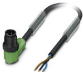
Sensor/Actuator cable, 3-position, PUR halogen-free, black-gray RAL 7021, Plug angled M12, A-coded, on free cable end, Cable length: 5 m, with plastic knurl
