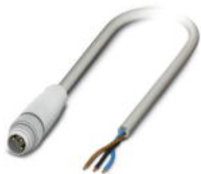
Sensor/Actuator cable, 3-position, PP-EPDM halogen-free, Gray RAL 7035, Plug straight M8, on free cable end, Cable length: 10 m, Hygienic design, with plastic knurl
