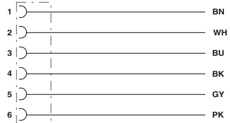
Contact assignment of M8 socket
