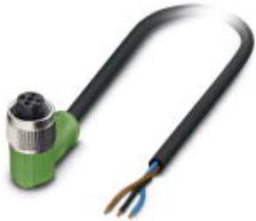
Sensor/Actuator cable, 3-position, PVC, Black RAL 9005, free cable end, on Socket angled M12, A-coded, Cable length: 10 m
