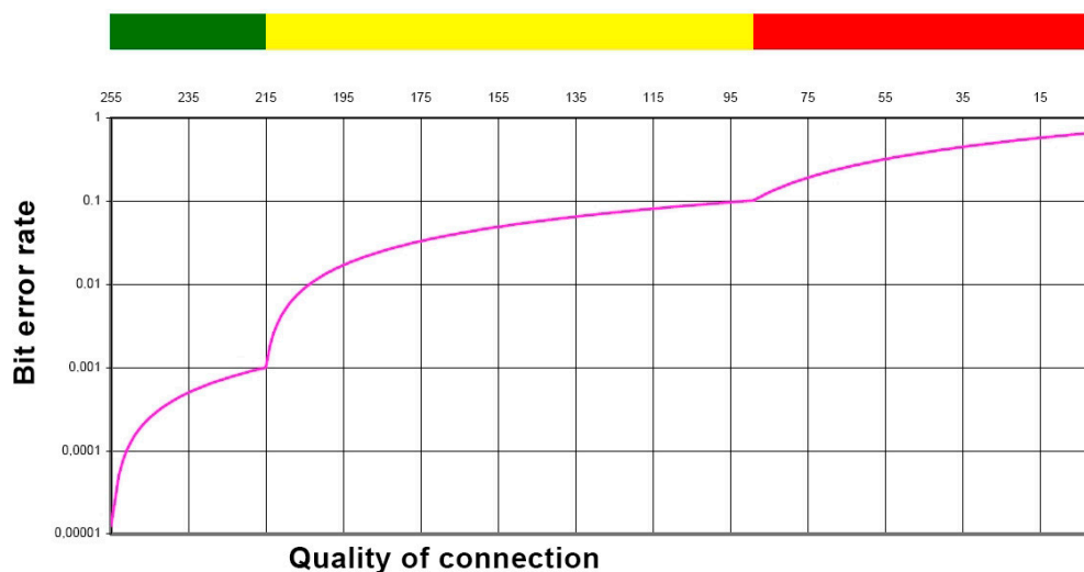
Figure 61: LED indication and connection between connection quality and bit error rate
