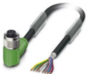
Sensor/Actuator cable, 8-position, PUR halogen-free, black-gray RAL 7021, shielded, free cable end, on Socket angled M12, A-coded, Cable length: 1.5 m
