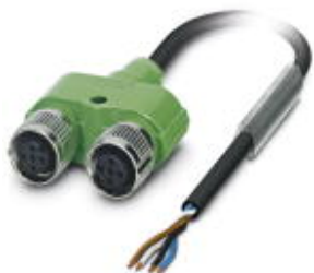
Sensor/Actuator cable, 4-position, PUR halogen-free, black-gray RAL 7021, free cable end, on Socket straight M12 SPEEDCON, A-coded and Socket straight M12 SPEEDCON, A-coded, Cable length: 5 m
