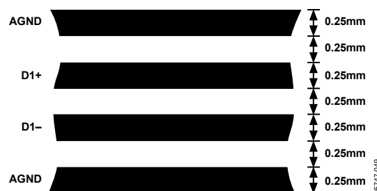
Figure 61. Arrangement of Signal Tracks
