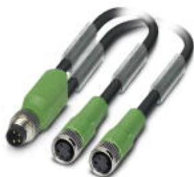
Sensor/Actuator cable, 3-position, PUR halogen-free, black-gray RAL 7021, Plug straight M8, on Socket straight M8 and Socket straight M8, Cable length: 0.6 m
