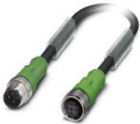
Sensor/Actuator cable, 4-position, PUR, black-gray RAL 7021, Plug straight M12, A-coded, on Socket straight M12, A-coded, Cable length: 10 m
