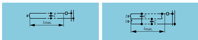
Figure 41: Two-wire control (left) and three-wire (pulsed) control
