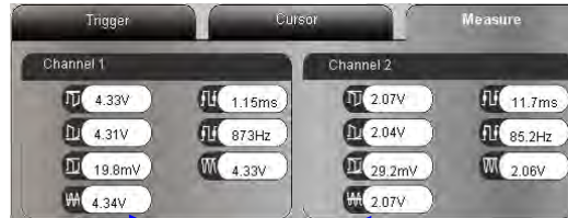
Figure 2-36: Resistor Voltage Measurements and Current Calculations ( Board of Education )
