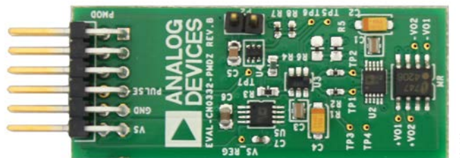
Figure 6. EVAL-CN0332-PMDZ Evaluation Board
