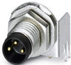
Sensor/actuator flush-type connector, connector, 3-pos. M8, rear/screw mounting with M8 fastening thread, with angled solder connection
