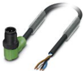
Sensor/Actuator cable, 4-position, PUR halogen-free, black-gray RAL 7021, Plug angled M12, A-coded, on free cable end, Cable length: 3 m, with plastic knurl
