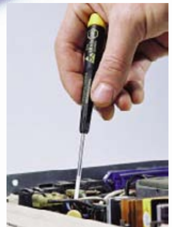
The rotating cap with contact area makes incremental adjustment quick and easy.
