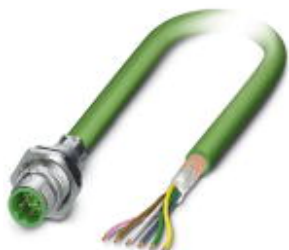
Bus system flush-type plug, INTERBUS, 5-pos., M12, shielded, B-coded, rear/screw mounting with M16 thread, with 2 m bus cable, 3 x 2 x 0.25 mm 2
