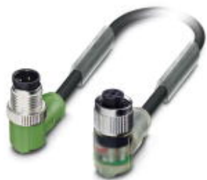
Sensor/Actuator cable, 4-position, PUR halogen-free, black-gray RAL 7021, Plug angled M12, A-coded, on Socket angled M12, A-coded, with 3 LEDs, Cable length: 1.5 m
