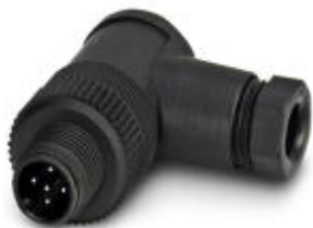
Sensor/actuator connector, male, angled, 5-pos., M12, A-coded, screw connection, plastic knurl, cable screw connection Pg7
